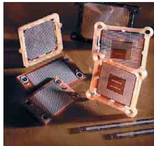
Рис. 1. MPI — Metallized Particle Interconnect
